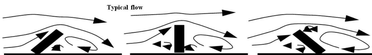
Figure 1: Shows attracting, deflecting and repelling spur dykes respectively from left.
